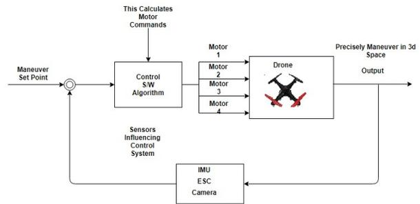
Figure 3. Control Parameters of the drone
