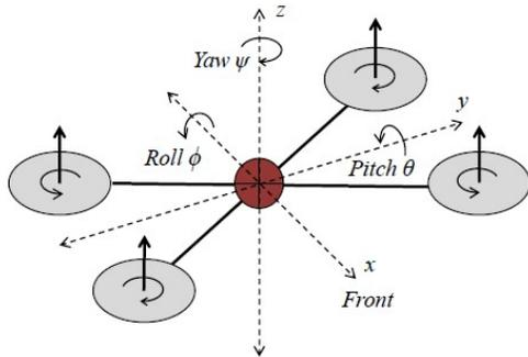
Figure 2. Control Parameters of the drone
