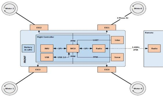
Figure 4. System Architecture
