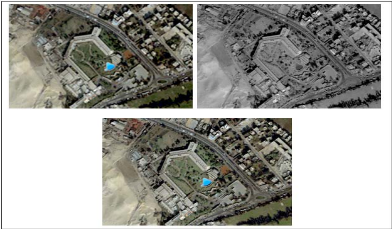
Figure. 2: Experimental Test Images over the Pyramid Area of Egypt in 2002. Quickbird Data MS and Quickbird PAN, Image Fused Resulted By SF Algorithm.
