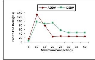
Figure 5. Maximum Connections vs End to end Delay
