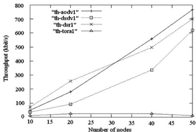
Figure 2: Throughput versus Number of Nodes (The Number of Nodes Is Smaller Than 50).
