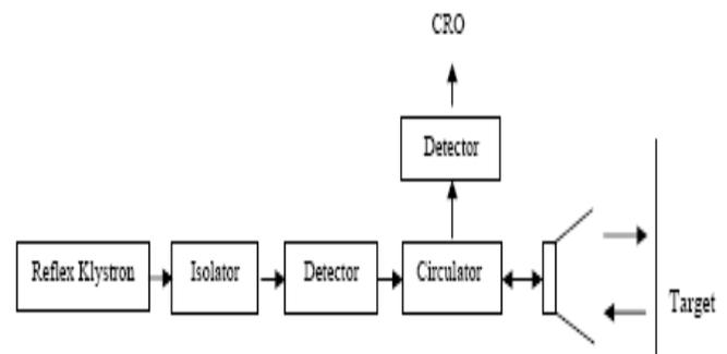
Figure.2. Block diagram of experimental set up.
