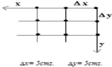
Fig.3. Grid for scanning
