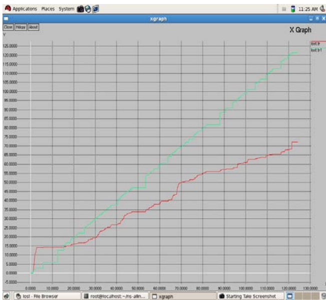
Figure 6: Comparison of loss rate for proposed system and simple wireless cluster sensor network
