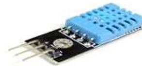
The digital temperature and humidity sensor DHT11 may be a combined sensor that consists of a computed signal which shows us digital measurement of temperature and humidity. It comprises 3 pins. Vcc(+5V) pin, Ground pin and data pin. The communication process will commence when the information line will emit start signals to DHT11, and DHT11 will receive the signals and return a solution signal.
