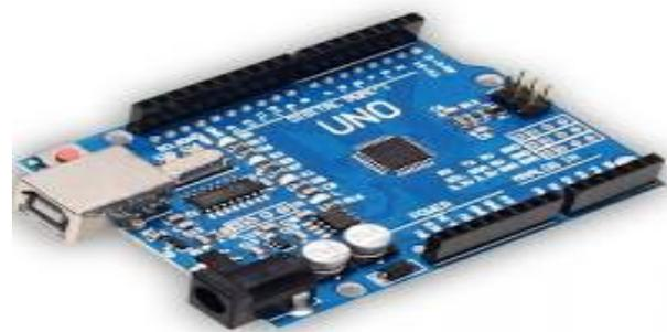
Fig : 1- Arduino Uno – microcontroller
