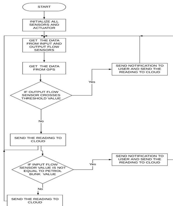
Figure 2: Flow Graph of Proposed Fuel Monitoring System
