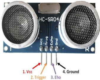
Figure 7: Ultrasonic Sensor
