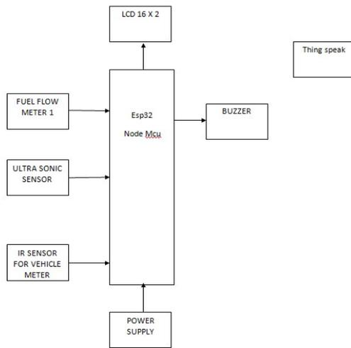
Figure 3:Block Diagram of Fuel Monitoring System
