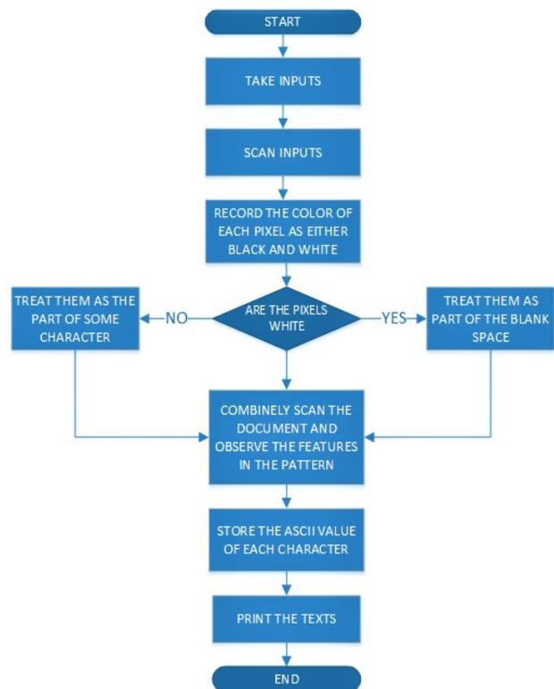
Figure 3. Inner Design and Working Principle of the proposed scanning application
