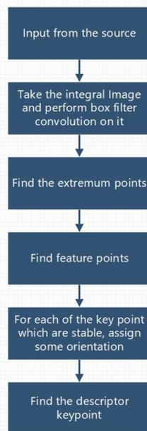
Figure 2. Feature detection Algorithm
