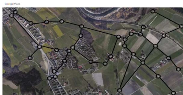
The above given figure shows the possible shortest path which is done by the suurballe's algorithm.
