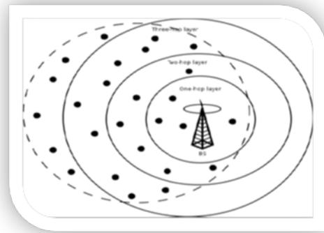
Figure 10: A three layer architecture
