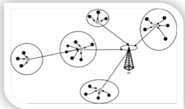
Figure 5: A LEACH-protocol-using network
