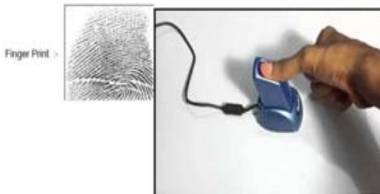
Fig. 1 Finger Print scanner
