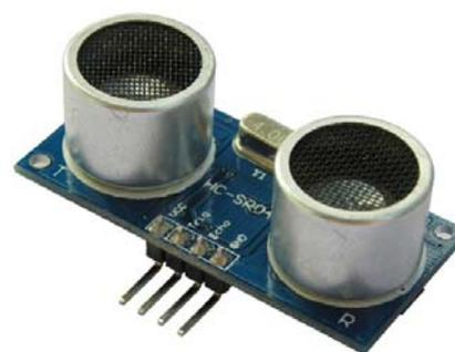
Fig. 1. Ultrasonic Sensor - HC-SR04
