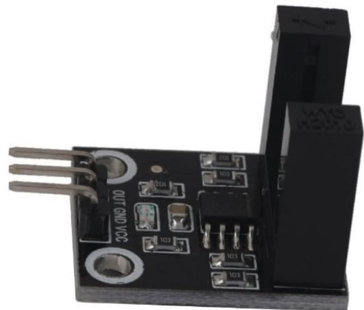
Fig. 5. Infrared Sensor
