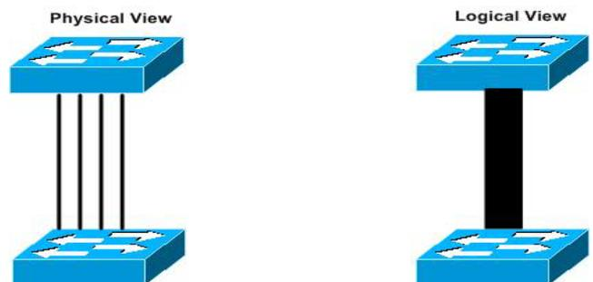
Figure 6 - Link Aggregation or EtherChannel,
