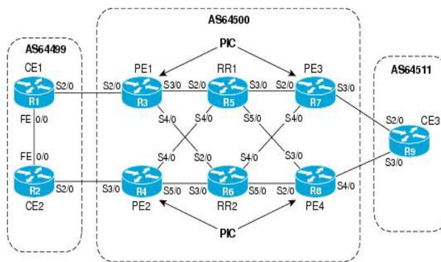
Figure 3 - BGP PIC for MPLS PE Primary-Alternate Scenario, Source - [http://www.cisco.com/c/en/us/td/docs/ios-xml/ios/iproute\\_bgp/configuration/xr-3s/irg-xe-3s-book/irg-bgp-mp-pic.html](http://www.cisco.com/c/en/us/td/docs/ios-xml/ios/iproute_bgp/configuration/xr-3s/irg-xe-3s-book/irg-bgp-mp-pic.html)
