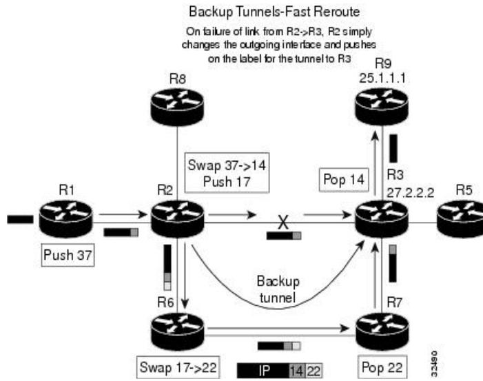
Figure 4 - MPLS FRR Mechanism,
