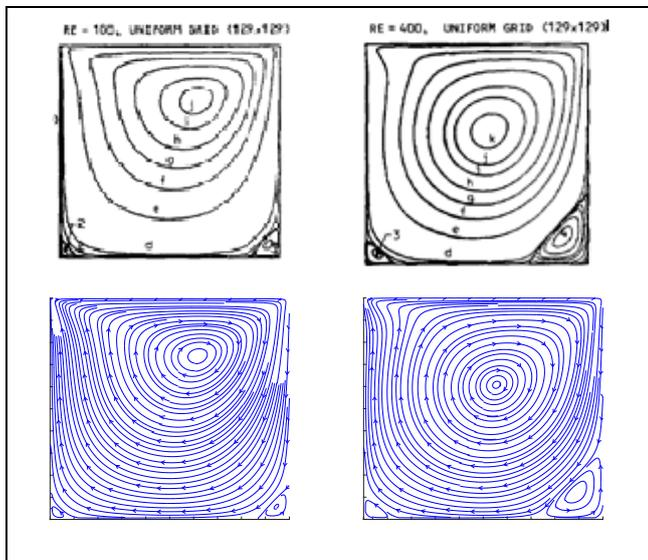
Fig. 2 Comparison of streamlines for our MAC method and results reported by Ghia et al. [5] for various Reynolds numbers
