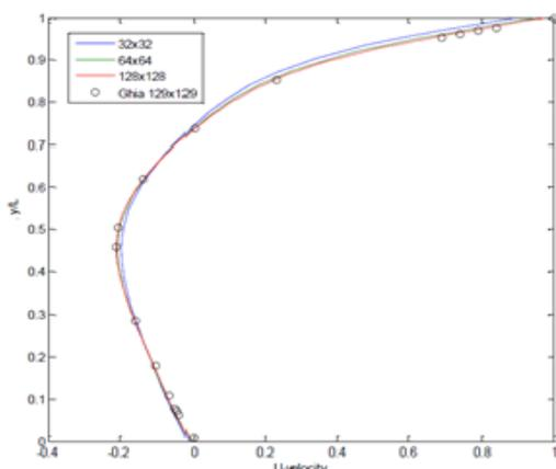
Fig. 3  $U$ -velocity profile along the  $y$ -axis through the geometric center of the square cavity ( $Re = 100$ ) with comparison to Ghia et al. [5].
