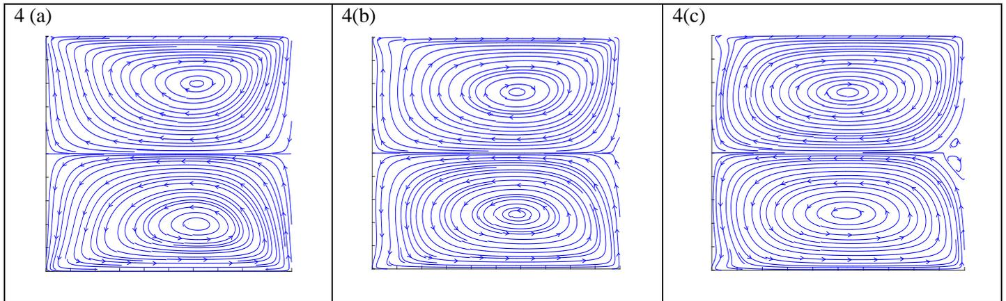
Fig. 4 Streamlines contours for different values of Reynolds number with horizontal walls are moving in same direction (a)  $Re=100$  (b)  $Re=400$  (c)  $Re= 1000$
