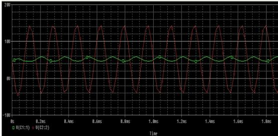
Figure 7: Transient Analysis of CB amplifier without EMI Signal
