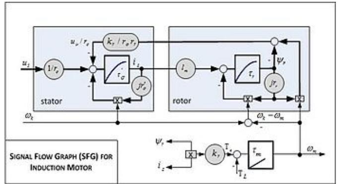
Fig 1 Signal flow Diagram of Induction Motor
