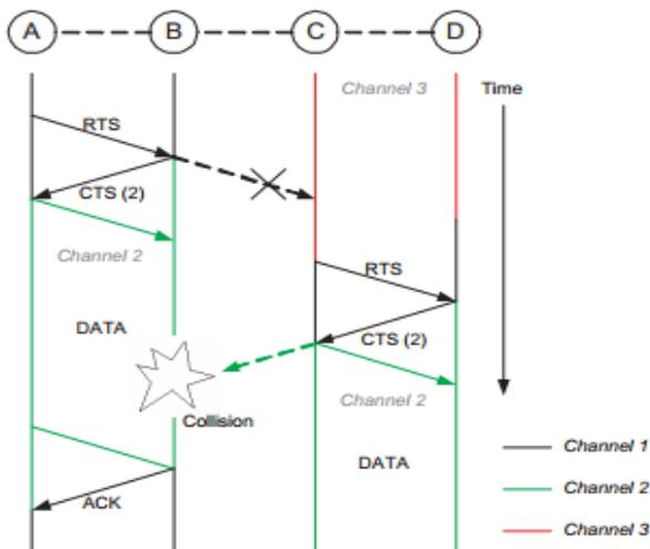
Fig.2.Multichannel hidden terminal problem. Channel is the control channel
