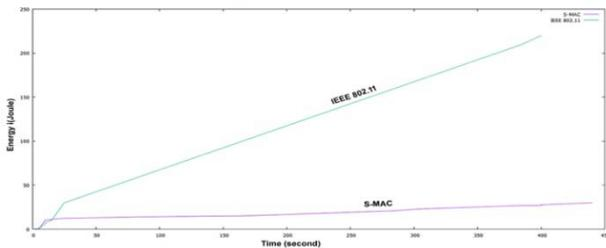
Fig.5. Energy Consumption at Intermediate Mode
