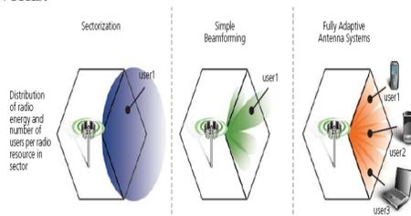
Figure 2. Beam Forming
