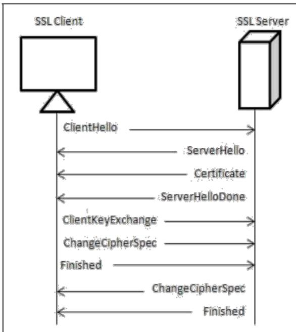
Figure 3:- Handshake and data transfer phases.
