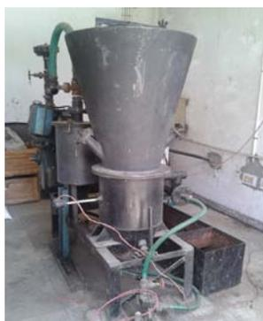
Figure-1 Dual Fuel Engine with Downdraft Gasifier setup
