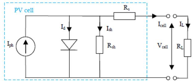
Figure 4. Equivalent Electrical circuit model of PV cells [37]
