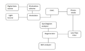
Fig 1: Inter-satellite Optical Wireless Communication (Is-OWC) System
