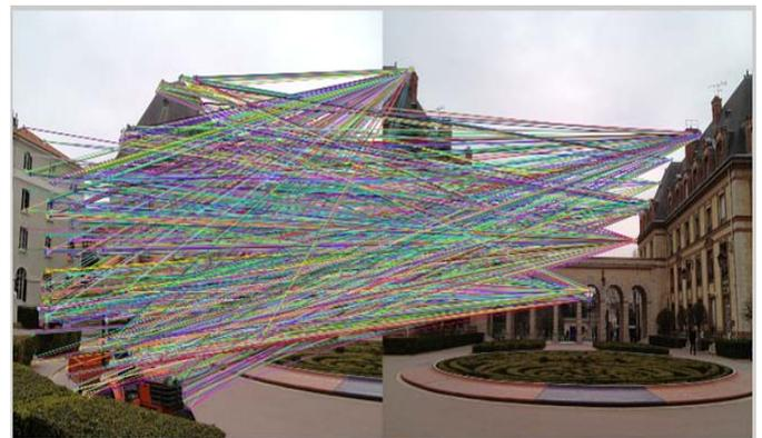
**Figure 7: Feature matching with RANSAC method**
