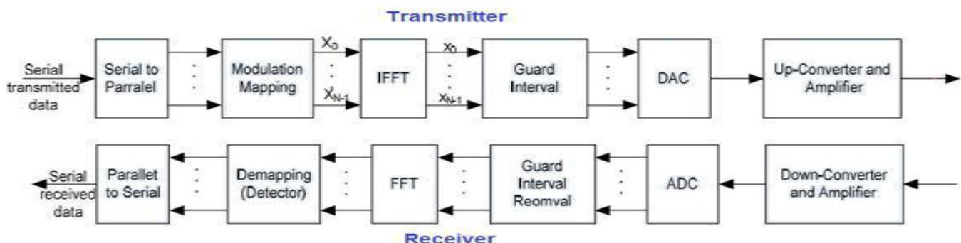
Fig.1.1 OFDM (orthogonal frequency division multiplexing). [19]
