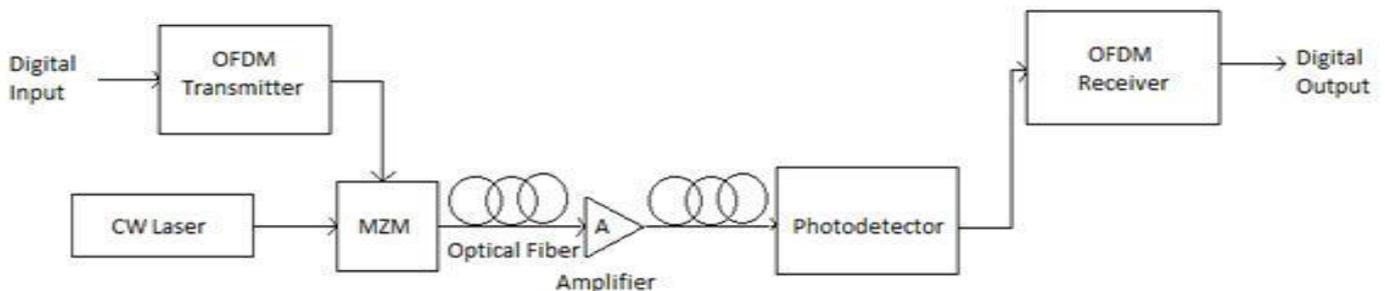
**Fig.3.1** Block diagram of OOFDM-ROF system. [11]
