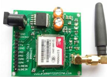
Figure 11 GSM Module
