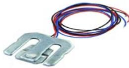
Figure 6 Load cell
