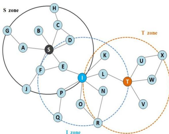
Figure2: A sample ZRP scenario for cloud based routing
