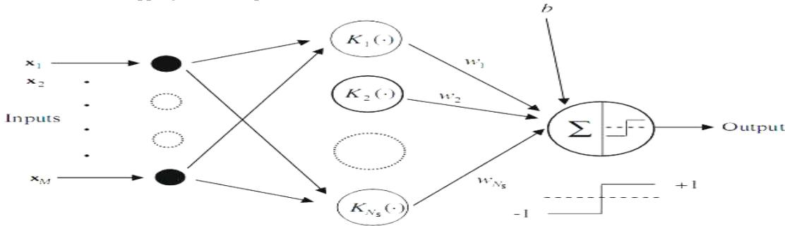
Fig. 4: Architecture of the SVM ( $N_s$  is the number of support vectors).
