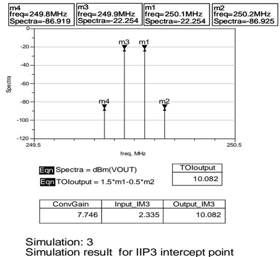
Figure.7 (b) Simulation for linearity.
