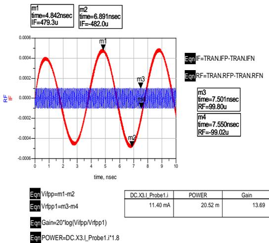
Figure.6 Voltage conversion gain.
