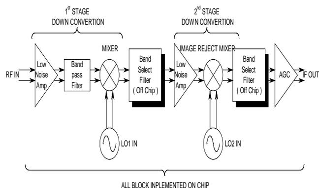
Figure. 1 Integrated Mixer block diagram
