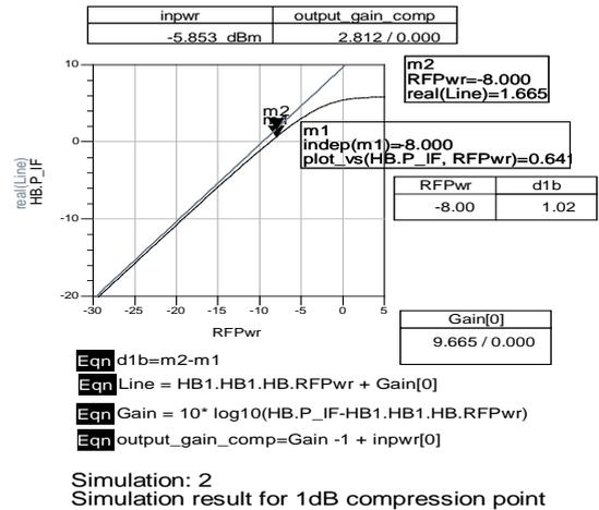
Figure.7 (a) Simulation for linearity.
