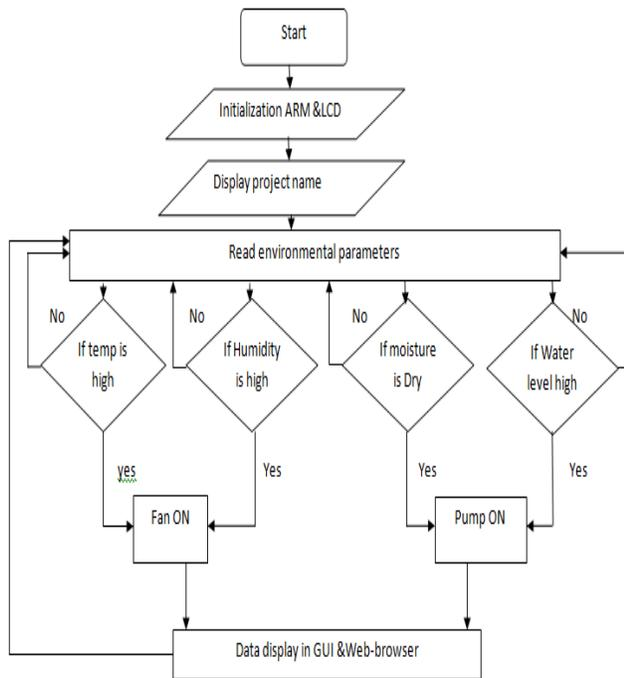
Fig 2: Flow chart of polyhouse automation
