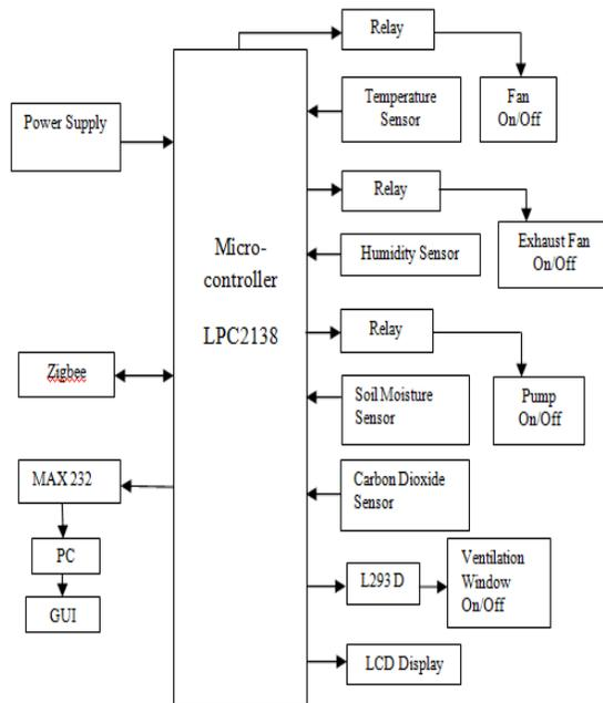
Fig.1.Block diagram of polyhouse automation
