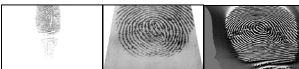
Figure 1. Fingerprint Patterns of a person taken using Optical Sensor "V300" by CrossMatch, Optical Sensor "U.are.U 4000" by Digital Persona, Thermal Sweeping Sensor "FingerChip FCD4B14CB" by Atmel respectively.
