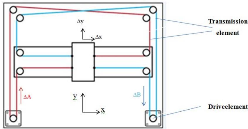
Fig 5:Core XY positioning principle diagram
