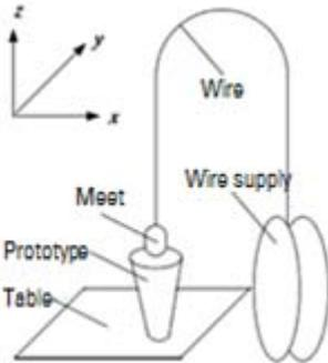
Fig 2: working principle of FDM 3D printer
