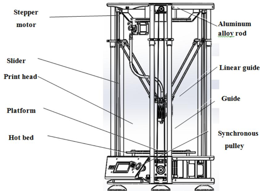
Fig 4: Schematic of parallel desktop 3D printer
