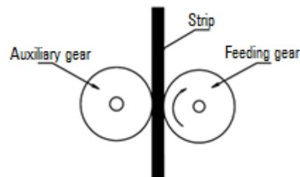
Fig 6: The principle diagram of the feeding device
