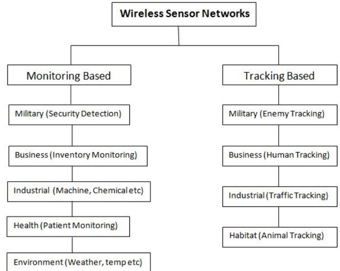
Fig.2. Applications of WSN based on monitoring and tracking
