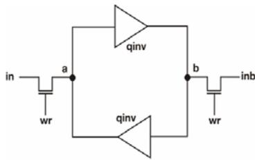
Figure 8: Block diagram representation of SRAM cell.
