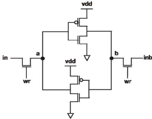
Figure 9: Circuit diagram representation of binary SRAM cell.
