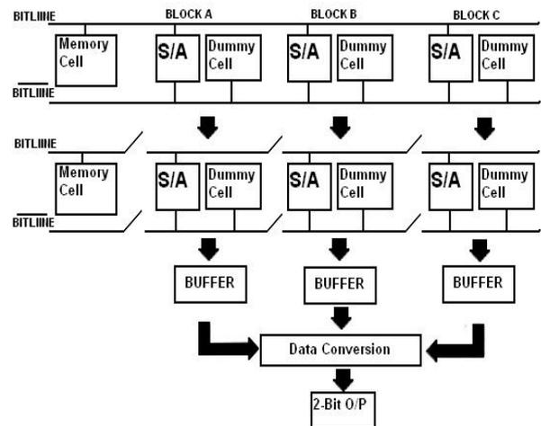
Figure 1: Parallel sensing scheme using globally generated reference voltage.
