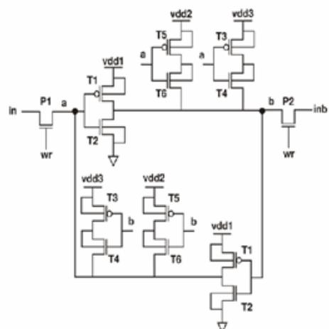
Figure 7: Gate level representation of Quaternary SRAM cell.
