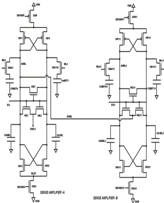
Figure 2: Proposed multilevel sense amplifier using sequential scheme.
