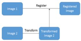
Fusion: consists in putting together information coming from different sources/data. This transformation is used to resample one data set.
