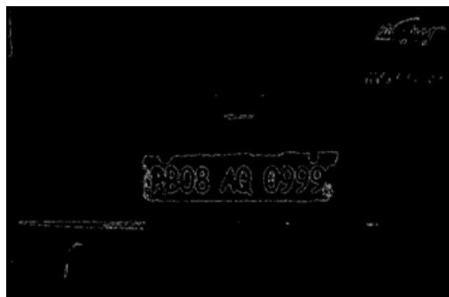
Figure.10: Edge Detection by Sobel operator
