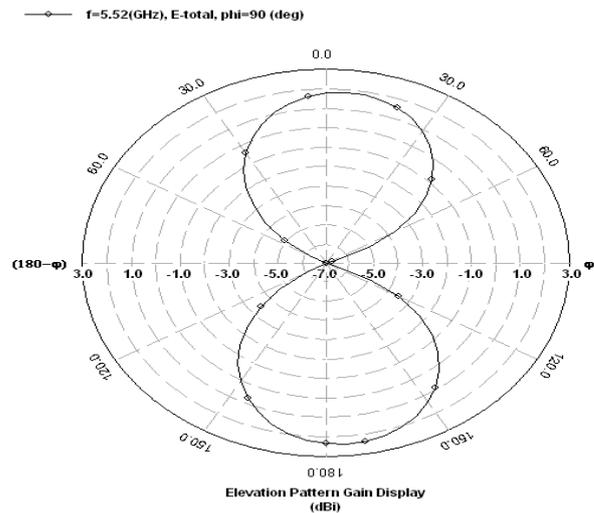
Figure 6(a): Elevation pattern at 5.52 GHz
