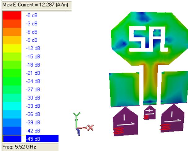
Figure 8: Current distribution of proposed Antenna at 5.52 GHz
