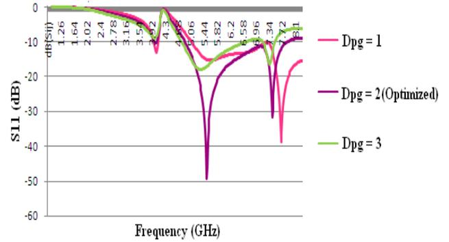
Figure 4: Effect of variation of  $D_{pg}$  on Antenna Performance
