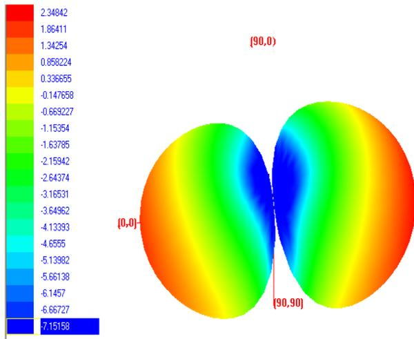
Figure 7: 3-Dimensional Pattern of Proposed Antenna at 5.52 GHz
