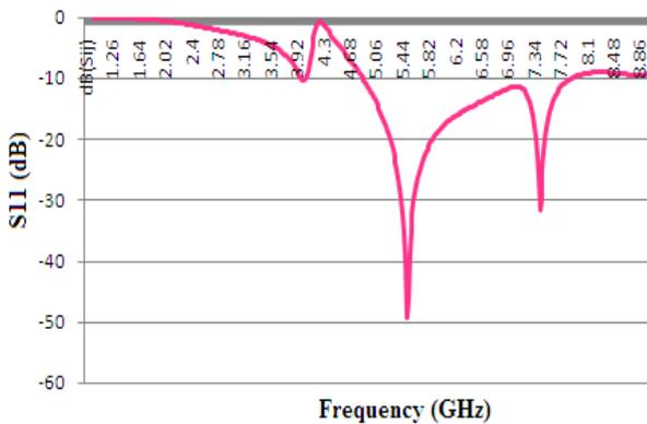
Figure 2: Return losses of proposed antenna
