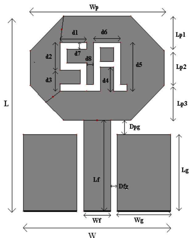
Figure 1: Geometry of proposed Antenna
