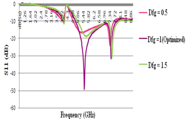
Figure 5: Effect of variation of  $D_{fg}$  on Antenna Performance
