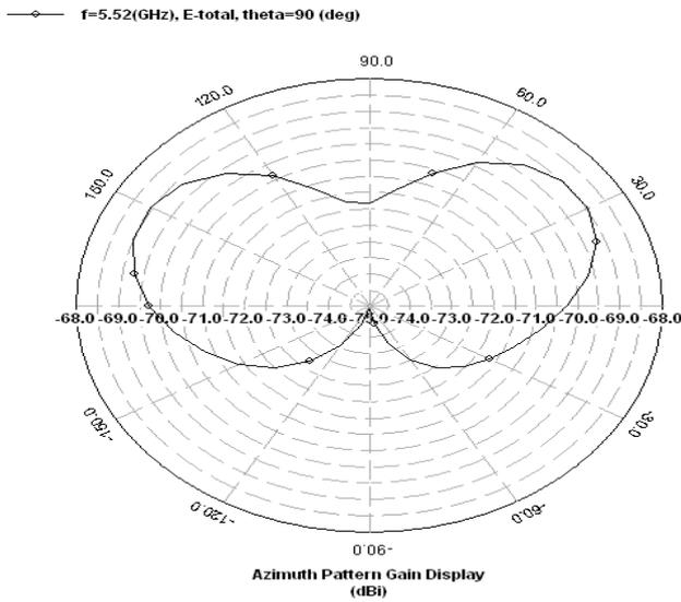
Figure 6(b): Azimuth pattern at 5.52 GHz
