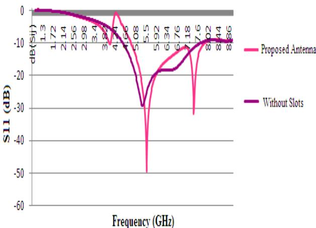
Figure 3: Effect of Slot Addition on Antenna Performance
