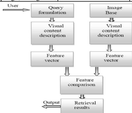
**Fig 1:** A Frame work of a CBIR System [10]
