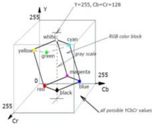
Fig.5 Representation of RGB colors in YCbCr
