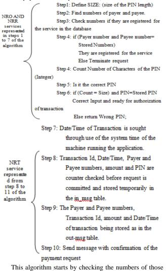
This algorithm starts by checking the numbers of those involved in the transaction, if they are registered or they are in the users database then the algorithm allows for the next step in the payment request to go ahead which is the payee's PIN is checked. If either one of the parties is not registered for the service then the request is terminated and an error message sent to the parties involved.
