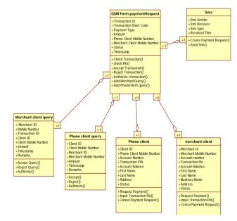
Figure 7: Class diagram
