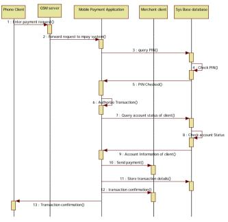
Figure 6: Sequence diagram showing the flow of information
