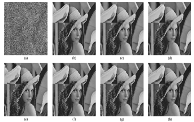
Fig. 4. Restoration results of different filters. (a) Corrupted Lena image with 80% salt-and-pepper noise (6.42 dB). (b) Original image. (c) CM filter (28.66 dB). (d) MMEM filter (27.66 dB). (e) AM filter (24.89 dB). (f) BDND filter (27.67 dB). (g) FM filter (23.08 dB). (h) AM-EPR filter (27.23 dB).
