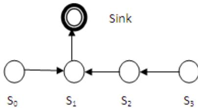
Some advantages of the PEGASIS firstly it can perform best than LEACH for different network sizes and topologies because it reduces formation of dynamic cluster in LEACH, and through the data chain data aggregation it decrease data transmission. Secondly energy load dispersed uniformly in the network.
