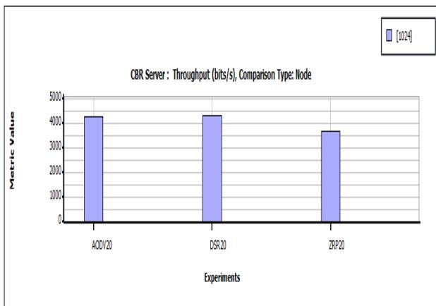
Figure 8 Throughput (bits/s) Vs 20 Nodes of RP
