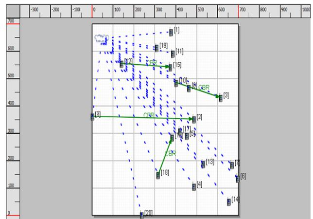
Figure 2 showing the nodes placement scenarios in this scenarios constant bit rate CBR apply from source nodes (9,10,12,18) to destination (2,3,15,16) in nodes placement scenarios.
