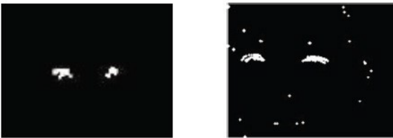
Left figure: example of eye contour pair returned by the original algorithm running on a desktop with a USB camera. The two white clusters identify the eye pair. Right figure: example of number of contours returned by EyePhone on the Nokia N810. The smaller dots are erroneously interpreted as eye contours.
