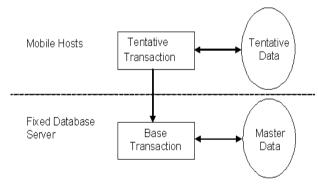
Figure 4 - Two-tier transaction model
