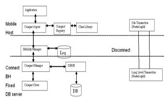
Figure 3- Pro-motion transaction architecture
