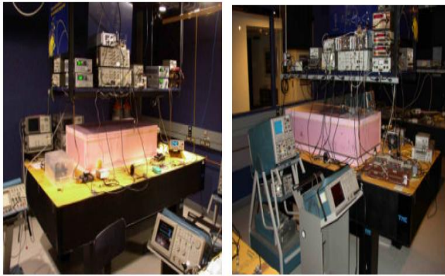
Figure 8. Physical layers of our weak-coherent link in the laboratory (Alice at left, Bob at right).
