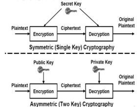
Figure 1: Symmetric and Asymmetric System Model
