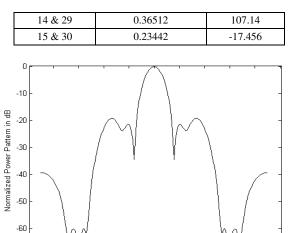
Fig.3. Normalized power pattern with wide null
