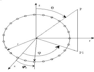
Figure.1. Uniform Circular Array of N isotropic elements
