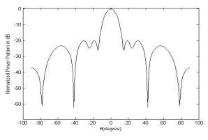
Figure.2. Normalized power pattern with multiple nulls
