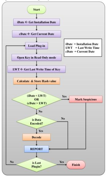
Figure 7: RegAnalyzer's Flowchart for processing registry
