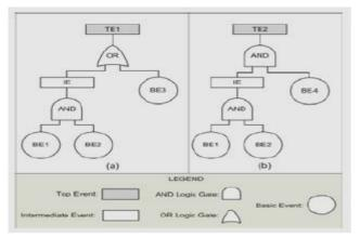
Figure 6. Fault tree structures with typical components
